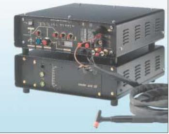
The Dual Arc 80 from Pro-Fusion supports both Micro-TIG and Micro-Plasma processes.
