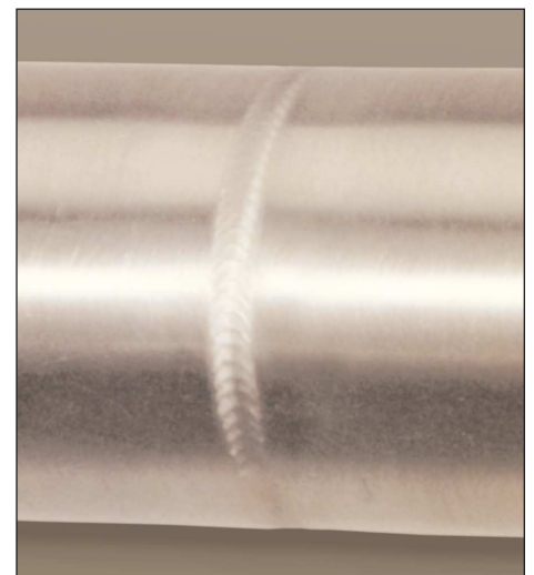
A typical orbital tube weld. Note the overlapping, pulsed-arc finish to the weld surface.
