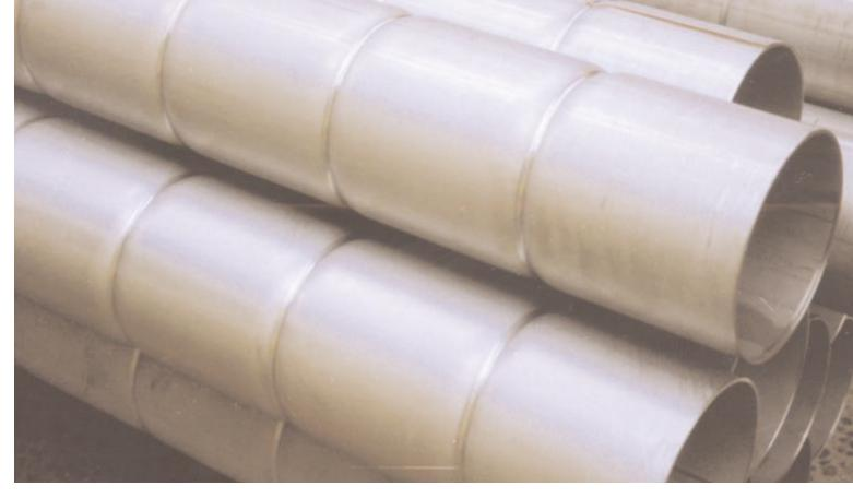
Naturally, with every benefit comes a drawback. A hydrogen addition is not suitable for welding all tube materials, especially some exotic alloys, because it can cause hydrogen embrittlement in the resultant weld. However, for the more commonly used stainless steels, there is no issue with embrittlement.
