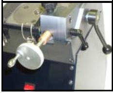
**Step 3**—Insert wand into cut-off fixture, move into enclosed cut-off wheel, flip open to get electrode.
