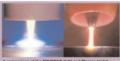
A comparison of the TIG/GTAW (left) and Plasma (right) welding arcs.
