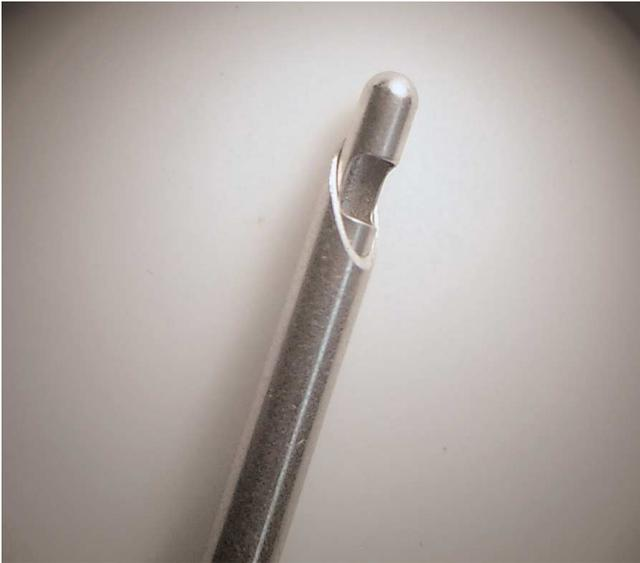
By imposing a welding arc for a controlled period of time, welders can close small diameter tubes to a perfect hemisphere.
