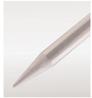
Figure 6 Using preground electrodes ensures that the electrode material quality, tip geometry, and ground electrode surface input to the welding process is constant.
