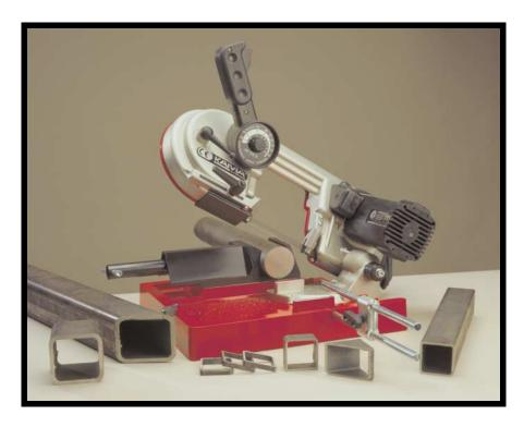
The Orbital Welding Benchtop Saw allows the user to make accurate, perpendicular cuts on parts up to 4 inches in diameter. When used with a tube squaring machine, this product makes up part of a precision preparation system for squaring tube and pipe prior to orbital welding.
