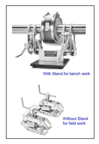
Accu-Fit helps welders complete flawless welds on tube and small diameter stainless steel pipe by ensuring precise alignment. Simply open the jaws with the parallel hand cranks, insert the tubes or pipes with any desired weld gap and then close the jaws - the Accu-Fit automatically concentrically aligns any two pipes within its range.
