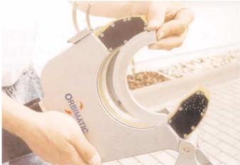
With a built-in integrated remote control in the rugged weldhead handle, all critical welding commands can be transmitted to the power source. This eliminates the need for an additional remote pendant.
